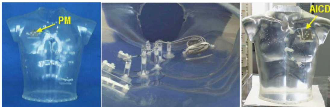
Fig. 6. Torso phantom used for the investigation. Left: torso for right pectoral implantation of pacemakers; Center: view from the bottom of the torso phantom of right pectoral implantation of pacemakers, the pacemaker and its electrodes—fixed by non metallic mounting pads—can be seen. Right: torso for left pectoral implantation of AICDs. [The color figure for this article is available online at www.interscience.wiley.com .]
