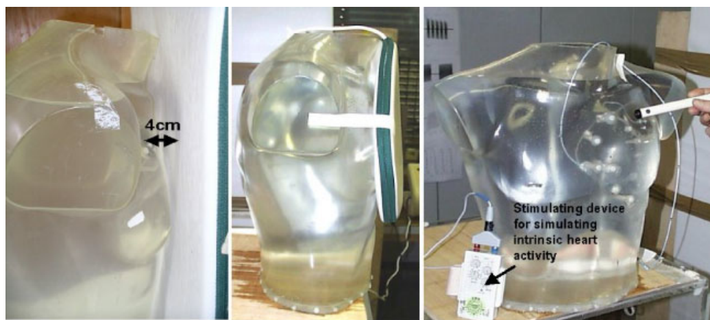
Fig. 7. Illustration of exposure situations using the whole body mat ( left ), the application cushion ( center ) and the bar applicator ( right ). In case of AICDs exposed by the bar applicator additionally proper detection of tachycardia during exposure was checked. [The color figure for this article is available online at www.interscience.wiley.com .]
